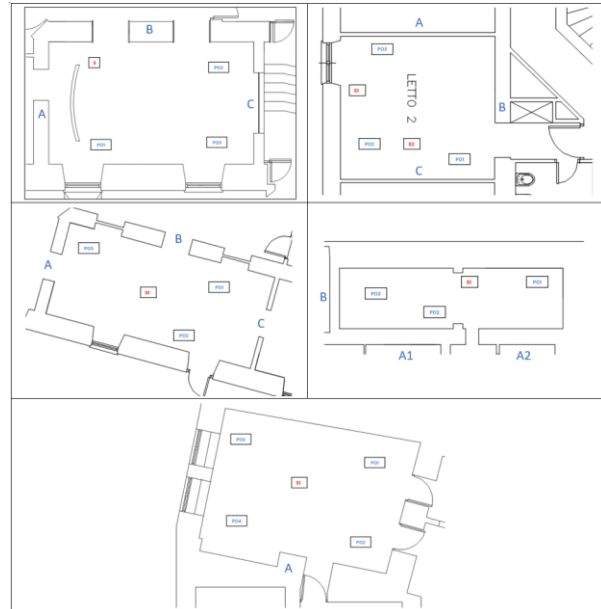
Figure 2. Planimetric representation of source point plan measurement points for T60 in the investigated rooms.
