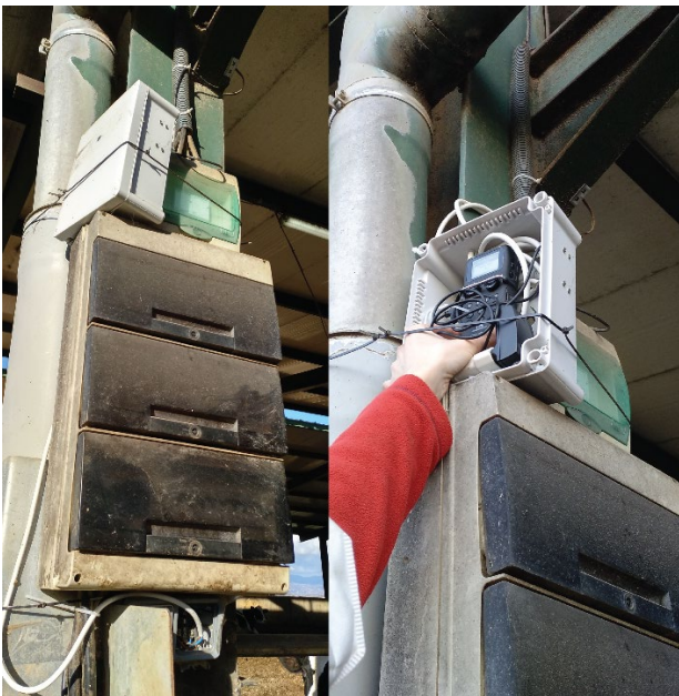
Figure 1 – Acoustical deployment sensor in farm (left), just above a light box, the recording box (right).
