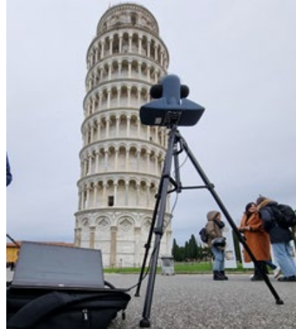
Figure 2. Photo taken at Point 4 during the soundwalk, using the Binaural Sensor Unit Code 1508 by HEAD Acoustics at the Tower of Pisa.
