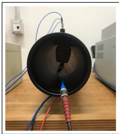
Figure 1. The test case: the plate and piezoelectric patch in the impedance tube.
