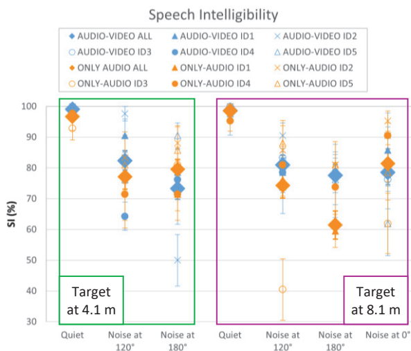
Figure 3. Average and standard error of the SI scores for all 7 scenes in case of AV and only audio test conditions for all subjects and for each single subject. Note that the mean distance from the 2 loudspeakers is considered as target distance.
