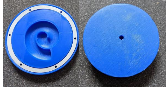
Figure 2. The reference metamaterial sound absorbing structure is used in measurements in impedance tubes.
