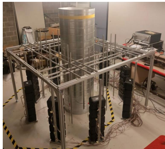
Figure 4. Small-scale DFAN setup for laboratory tests.
