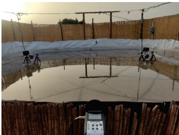
Figure 1. Experimental set-up: pond filled with water with two pairs of loudspeakers and vibratory devices.
