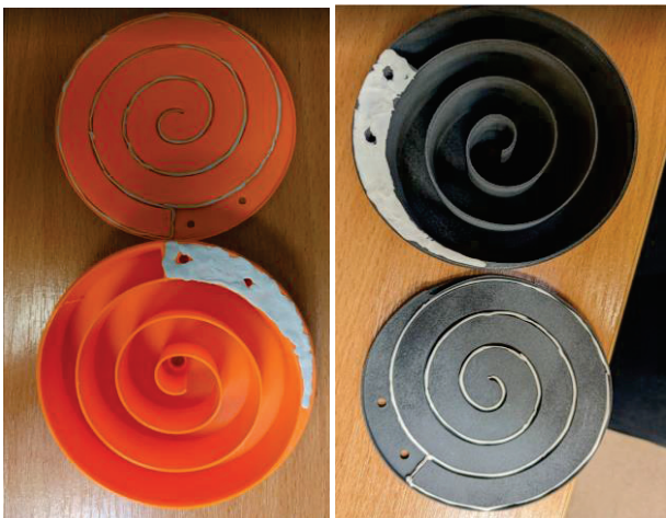
Figure 2. Selected 3D prints in FDM (left) and SLS (right) with sealing
