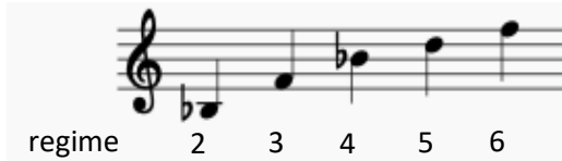
Figure 2. Notes corresponding to the five different regimes simulated on a Bb trumpet.
